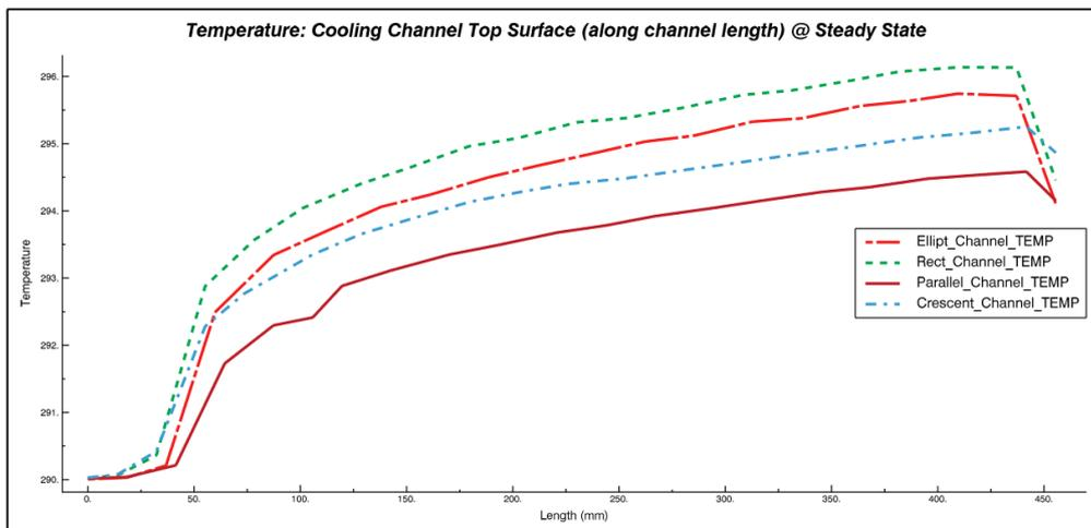
Figure 5. Channel top surface temperature comparison
