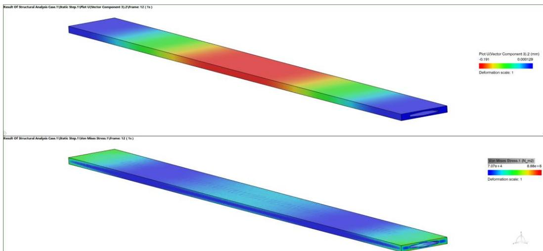
**Figure 10. The optimized vertical deformation and von-mises stress contours**
