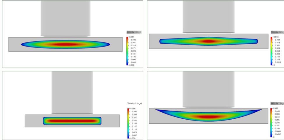
Figure 4. Velocity contours at outlet in different cross-section designs
