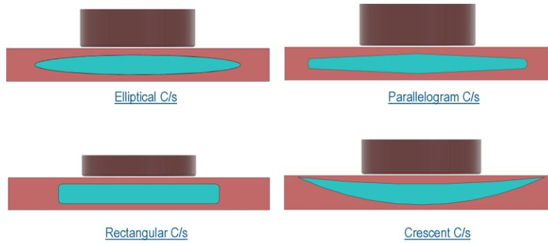
**Figure 2. Cross Section Configurations**
