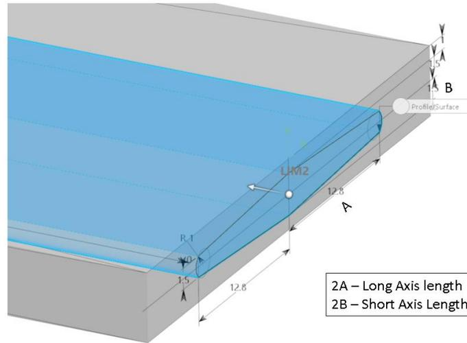
**Figure 6. Parameterized channel cross-section for the fluid volume (blue)**
