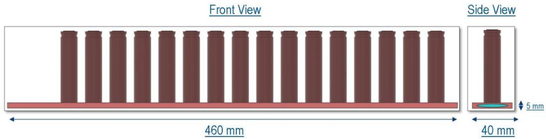
**Figure 1. Fluid channel model with battery cell**
