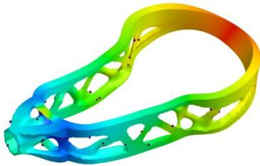
The flow front is shown at various stages of the fill process similar to molding a 'short shot' where the filling phase is stopped midway through the injection molding as a diagnostic tool.
