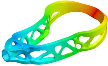
The full simulation shown below agrees fairly well with the initial prediction and can be seen below. Undesirable air traps shown at the dot locations.
