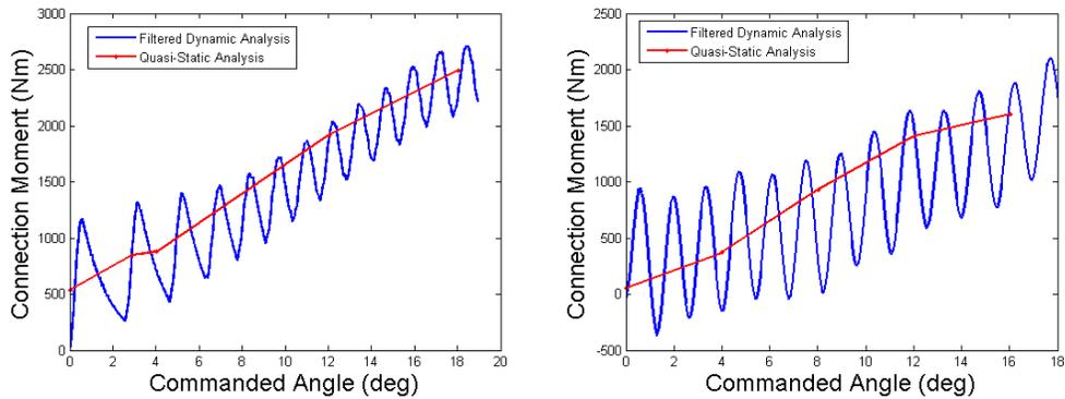
**Figure 12. Results of the dynamic analysis after a low-pass filter of 30 Hz is applied are compared to quasi-static results both with free play (left) and without free play (right).**
