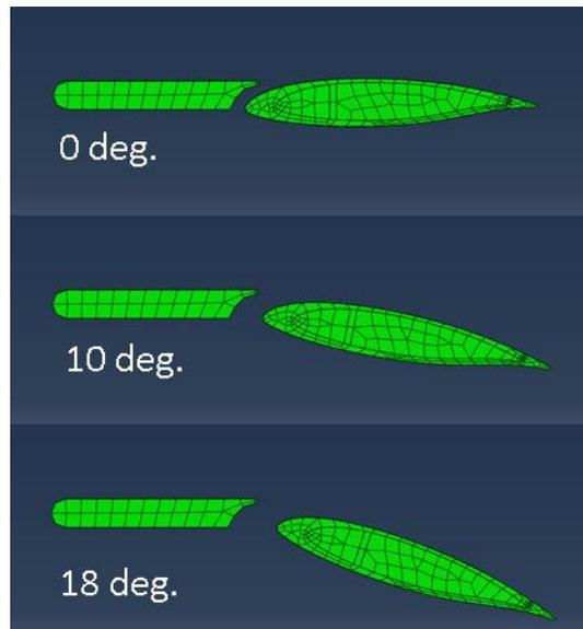
Figure 2. Three commanded deployment angles for the slat/flap system are depicted:  $0^\circ$ ,  $10^\circ$ , and  $18^\circ$ .
