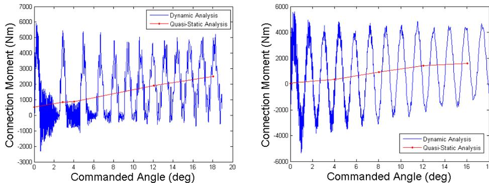
**Figure 8. The results comparing dynamic (blue) and quasi-static (red) analyses. Left: one degree of free play is included. Right: no free play is included.**
