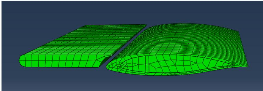
**Figure 3. The FEM mesh was largely composed of continuum elements, with shell elements on the flap sides.**
