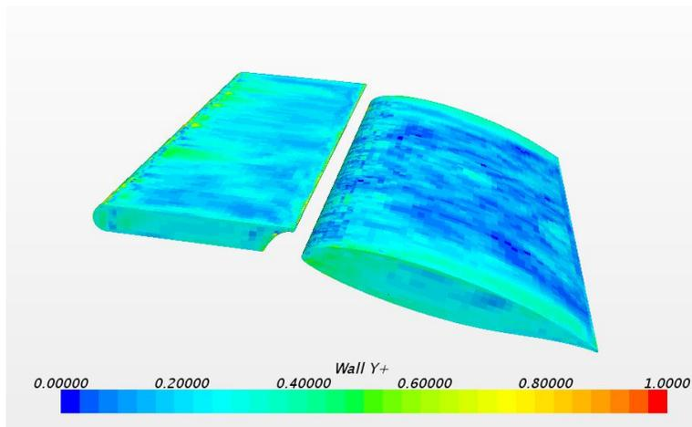
**Figure 7. Wall  $y^+$  values indicate appropriate initial wall spacing ( $y^+ < 1$ ).**
