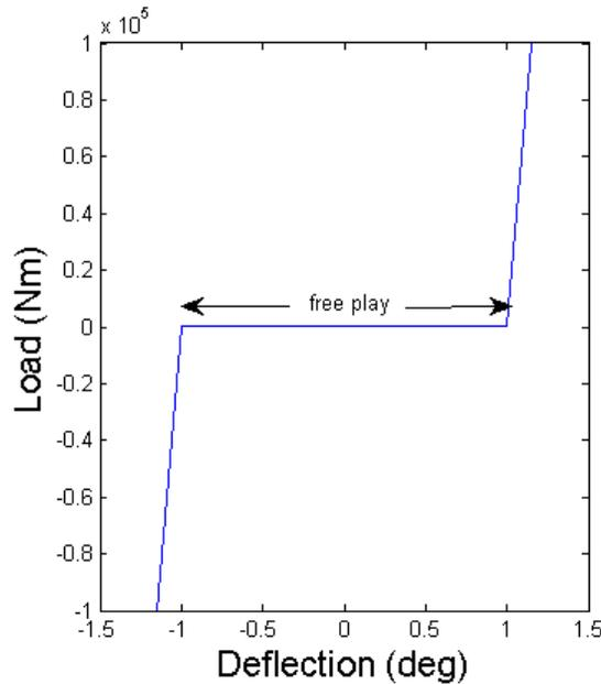
**Figure 5. Free play was modeled as a region where a change in deflection could be obtained without maintaining a supporting load.**
