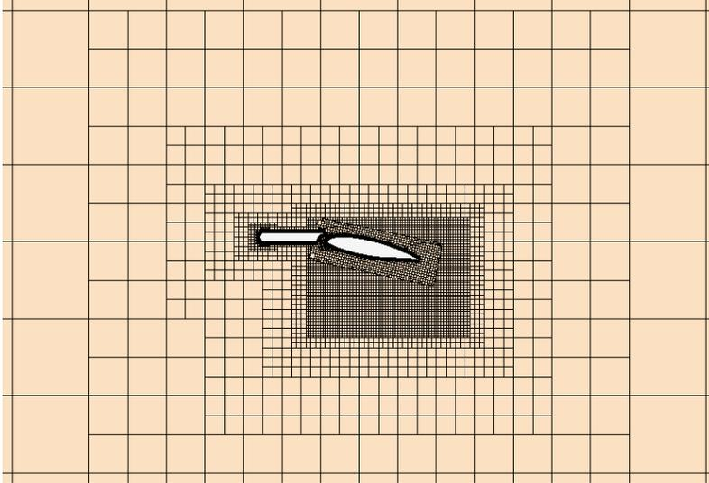
**Figure 6. The CFD domain was composed of two overset meshes. The large background mesh contains the leading slat while the flap is contained in the small overset mesh.**
