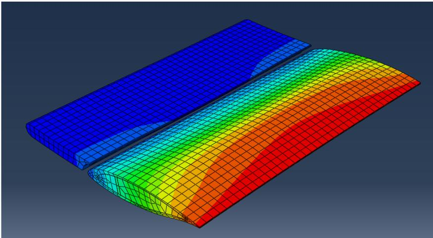
**Figure 11. The first mode of the demonstration case when no free play is included.**
