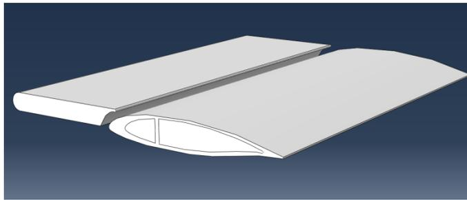
Figure 1. The geometry of the case considered consists of a leading slat and a trailing flap.
