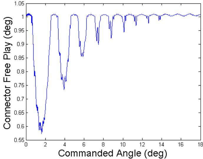
**Figure 9. The actuator connector angle as a function of commanded angle.**
