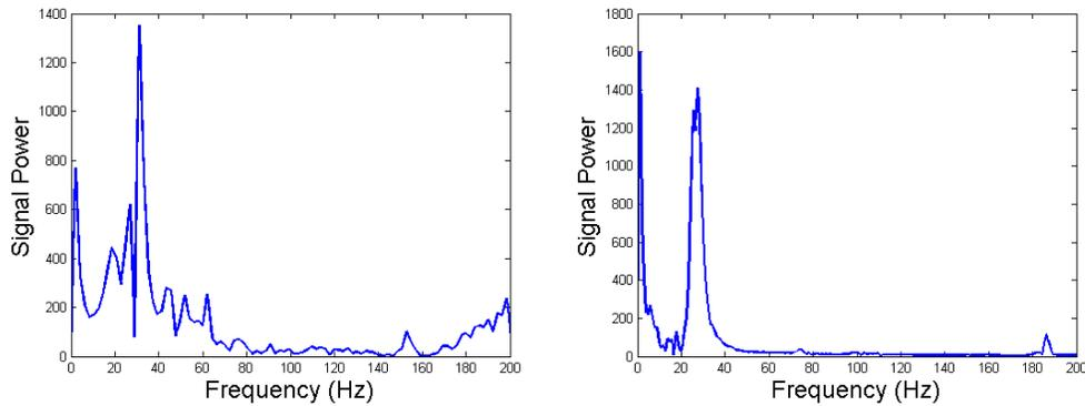
**Figure 10. Frequency response of the dynamic analysis with free play (on left) and without free play (on right).**
