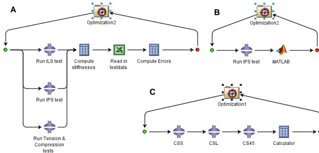
**Figure 1. Isight simflow for the optimization of A) linear stiffness properties, B) non-linear resin properties, and C) compressive fiber failure properties.**
