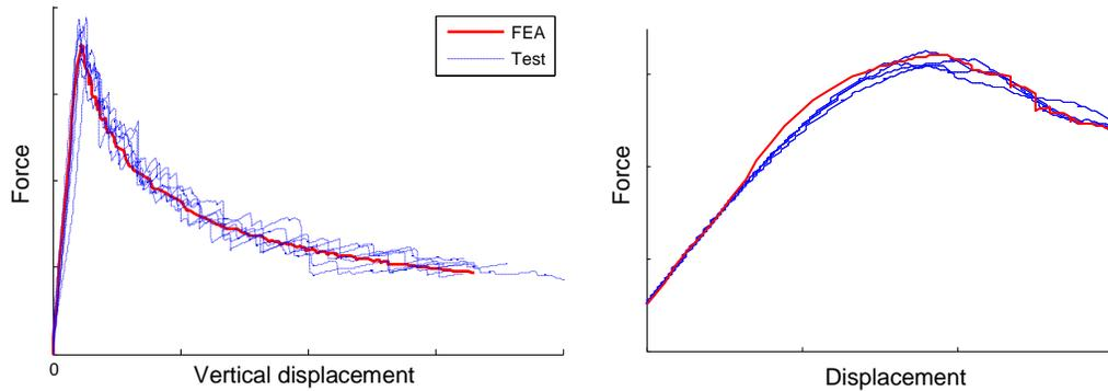
**Figure 7. Left) Force-displacement graph of peel test, Right) Force displacement graphs of 3 point bending test ILS3 (blue=no damage; red=failed).**
