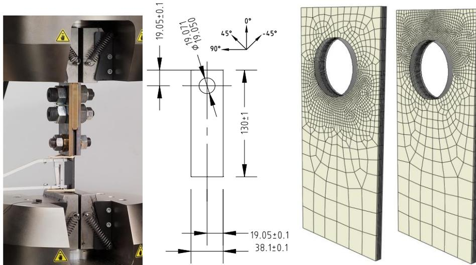
Figure 4. Left) Photograph of bearing compression test setup; Middle) Dimensions; Right) FEA mesh (left: compression; right: tension).
