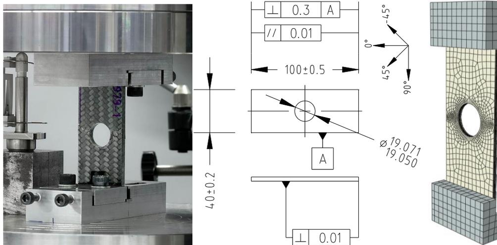
Figure 5. Left) Photograph of open hole compression test setup; Middle) Dimensions; Right) FEA mesh.
