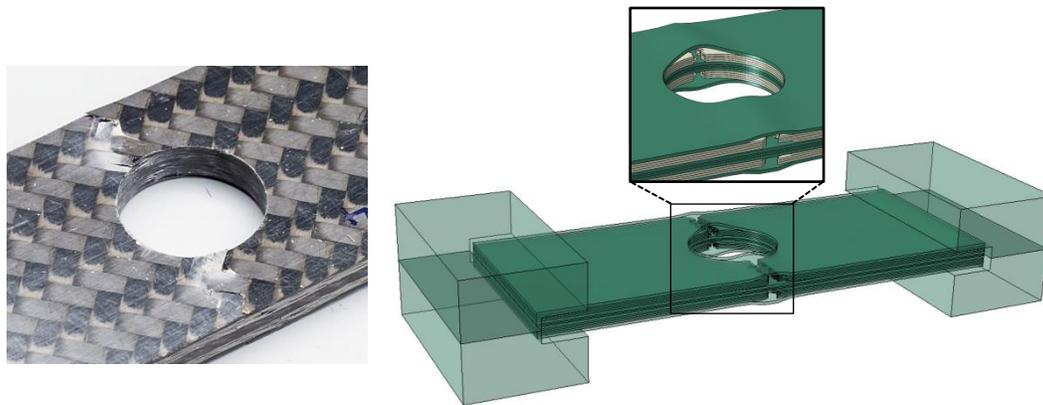
**Figure 8. Left) photograph of failed open hole compression test specimen, Right) Deformed FEA model after failure**
