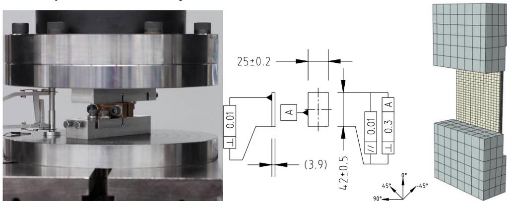
Figure 3. Top-Left) Photograph of compression test setup; Middle) Dimensions; Right) FEA mesh.
