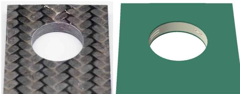
**Figure 10. Left) photograph of failed bearing tension test specimen, Right) Deformed FEA model after failure**
