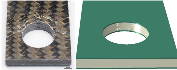
**Figure 9. Left) photograph of failed bearing compression test specimen, Right) Deformed FEA model after failure**
