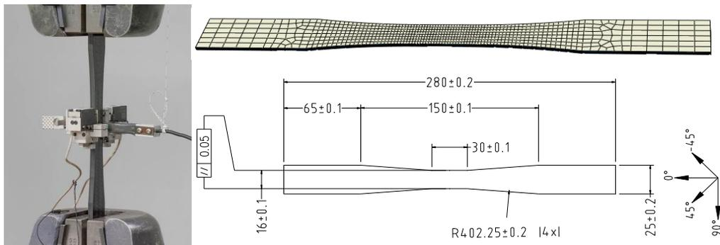
Figure 2. Top-Left) Photograph of tensile test setup; Top-Right) Dimensions; Bottom) FEA mesh.
