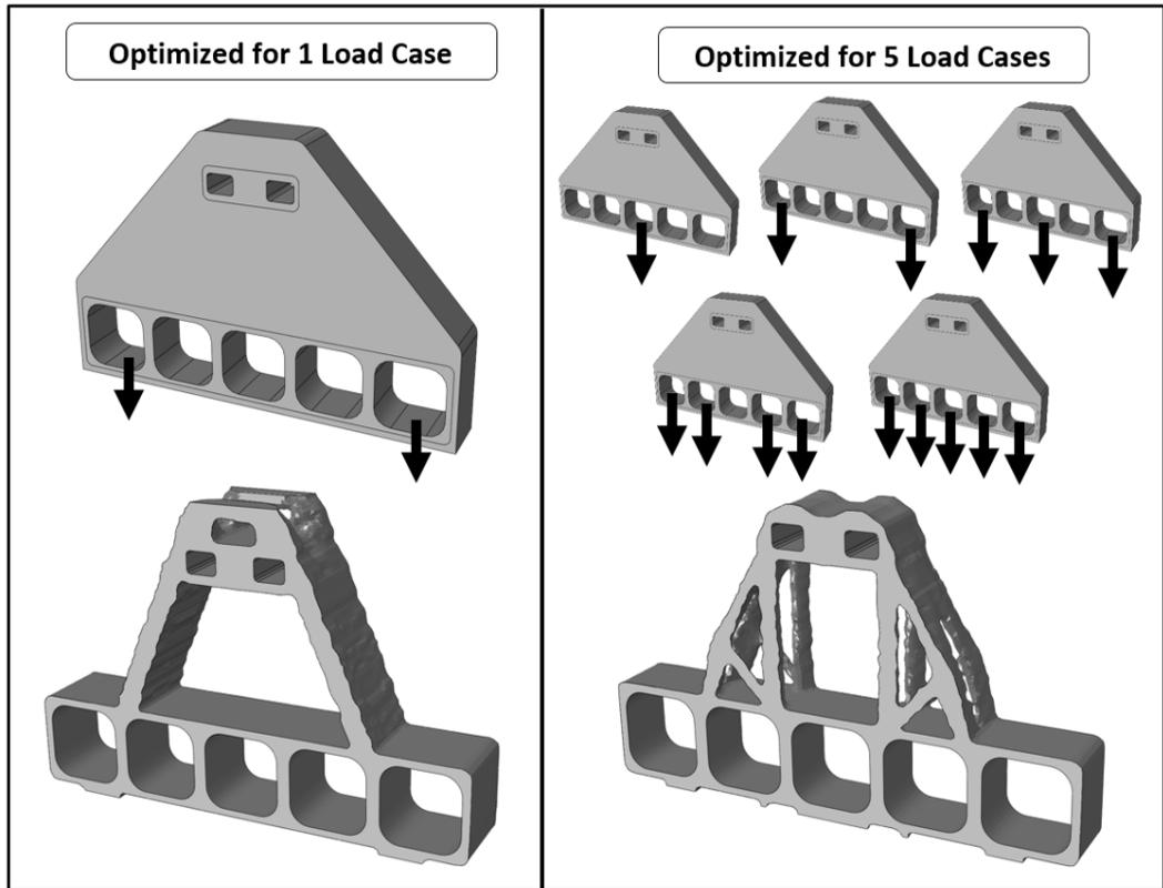
**Figure 2. Results for optimizing hanger for 1 load case (left) vs optimizing hanger for 5 load cases (right)**
