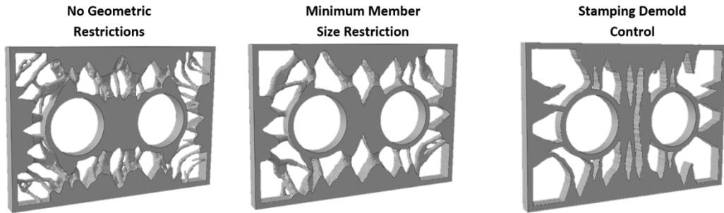
**Figure 5. Optimized plate using different geometric restrictions**
