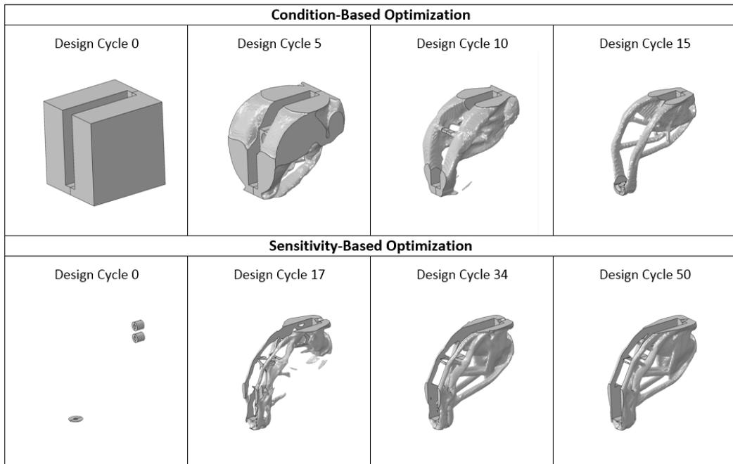
**Figure 3. Design iterations for bracket using Condition-Based (top) and Sensitivity-Based (bottom) algorithms**
