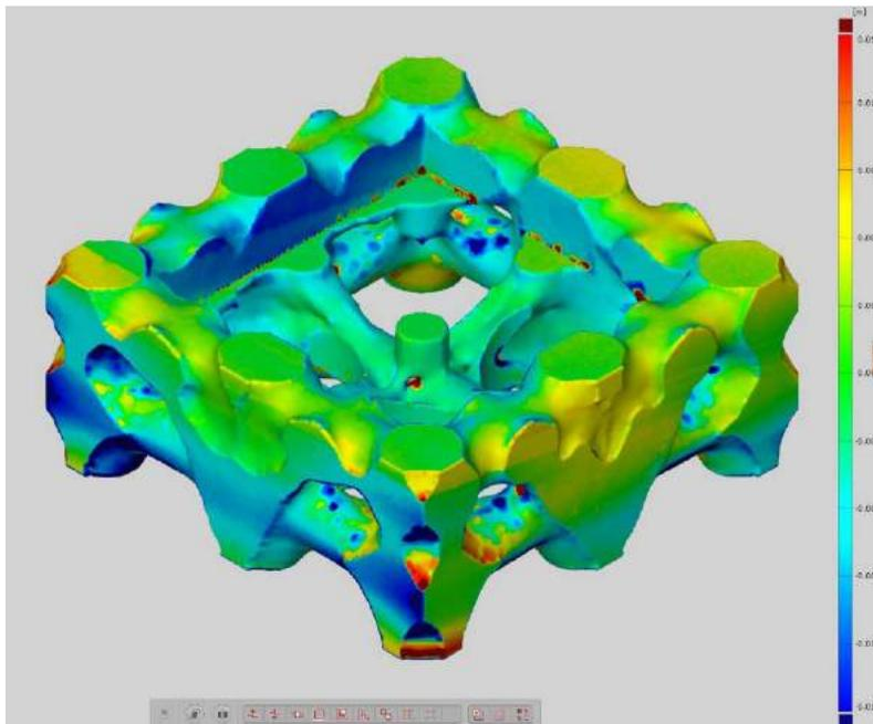
**Figure 6. GOM ATOS III Triple Scan results for AM part overlaid on original part file showing tolerance discrepancies**
