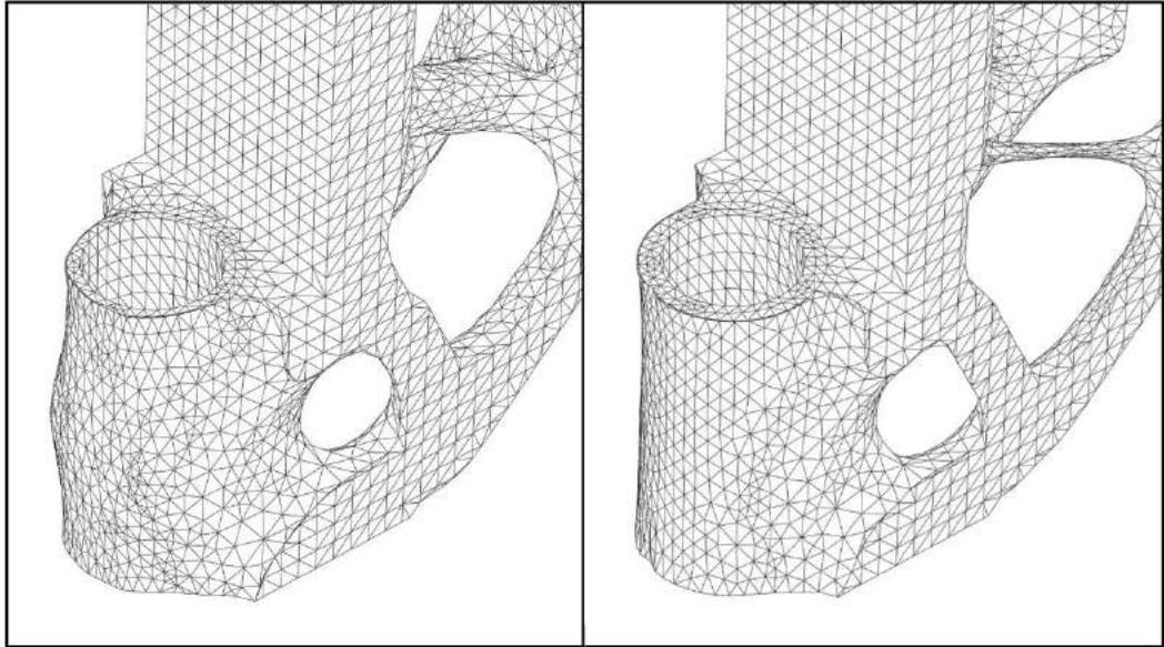
**Figure 4. Freezing only hole face (left) vs. freezing a cell surrounding hole (right)**
