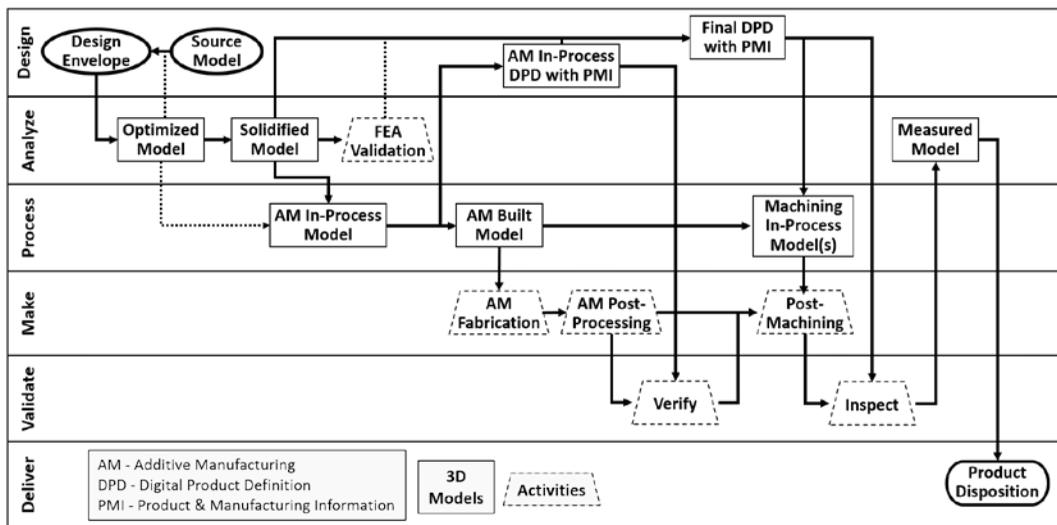
**Figure 1. Novel workflow created for using topology optimization to design for additive manufacturing**
