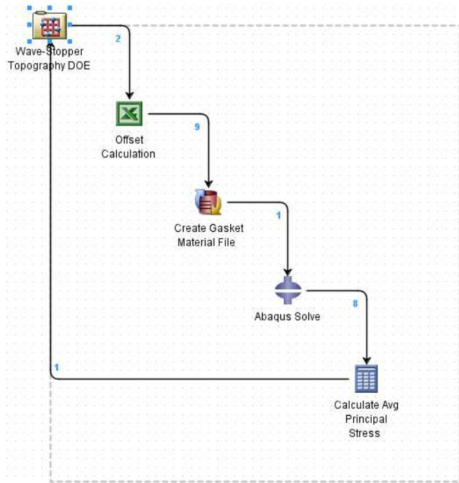
**Figure 9. Stopper topography DOE dataflow**
