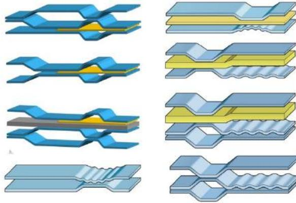
**Figure 3. Multi-layer gasket design options**
