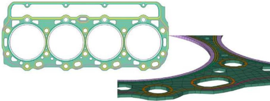
**Figure 4. Model with gasket elements**
