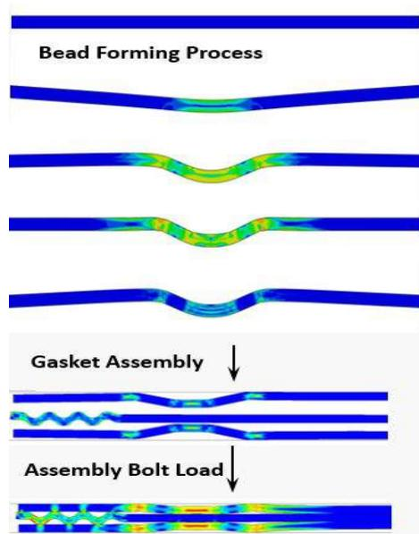
**Figure 12. Loading steps for fatigue analysis**
