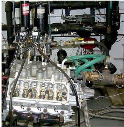
**Figure 15. Pulsator test configuration**
