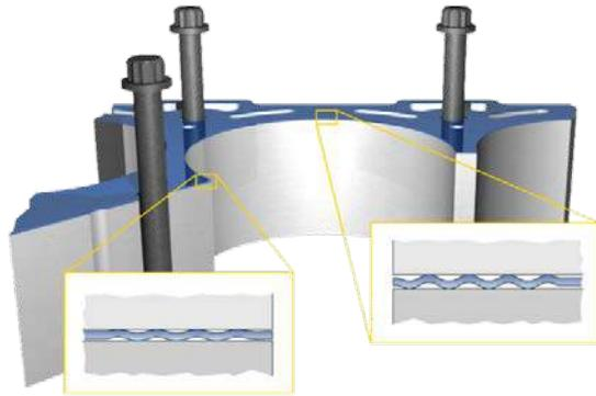
**Figure 8. Varying stiffness behavior of the Wave-Stopper™**
