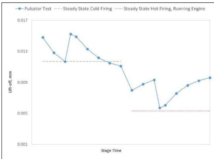
**Figure 16. Lift-off results from the Pulsator test versus steady state thermals**
