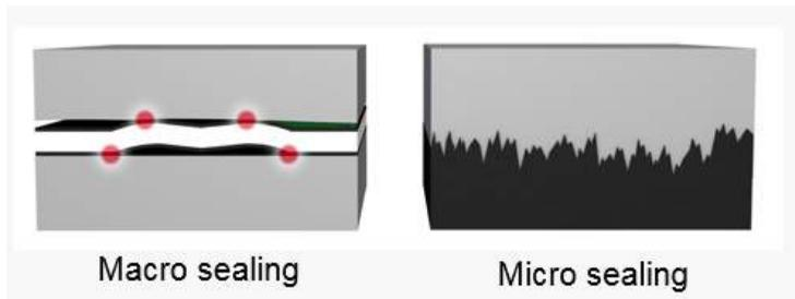
Figure 2. Two sealing functions of the gasket
