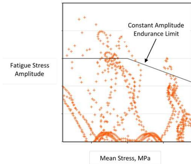
**Figure 14. Stress amplitude versus mean stress plot (Haigh Diagram)**
