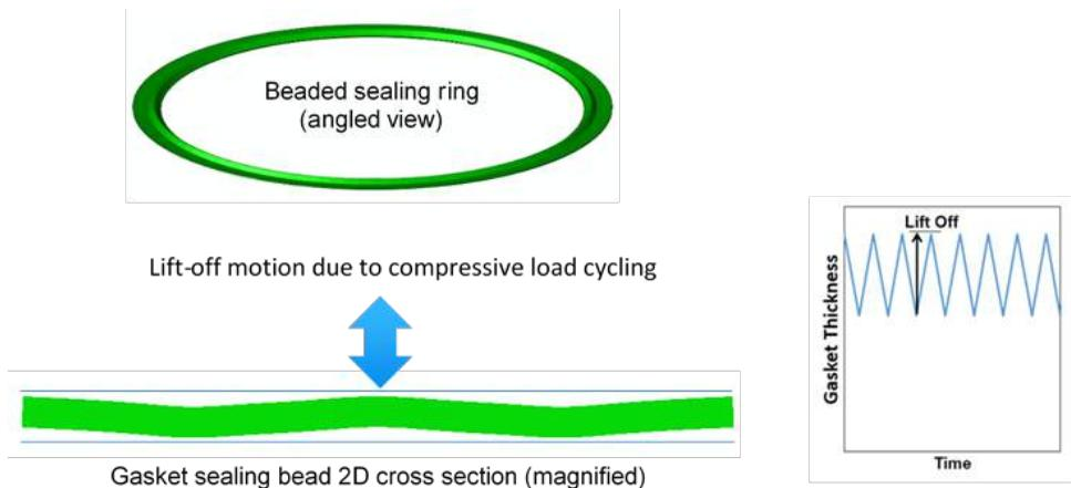
**Figure 11. Gasket fatigue test configuration**
