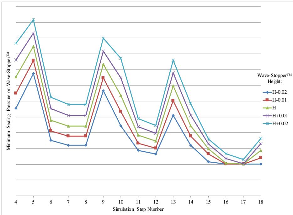
**Figure 7. Wave-Stopper™ sealing pressure results**
