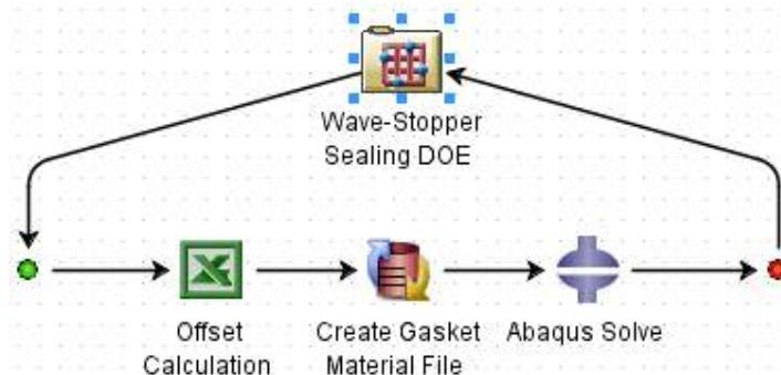
**Figure 6. Wave-Stopper™ sealing pressure DOE sim-flow**
