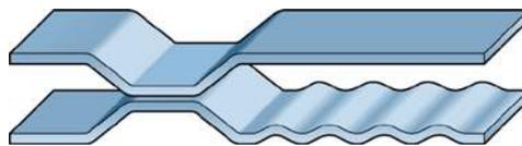
**Figure 5. Wave-Stopper™ combustion seal**
