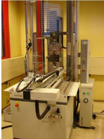
**Figure 11. Automated tensile testing equipment (DuPont ETC, Geneva)**
