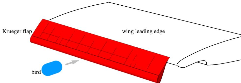
**Figure 2. Krueger flap concept treated in this study.**
