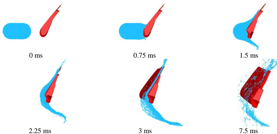
**Figure 6. Cross-sectional view of bird strike on Krueger flap.**
