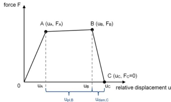
Figure 5. Illustration of elastic, plastic and damage behaviour of fastener element.
