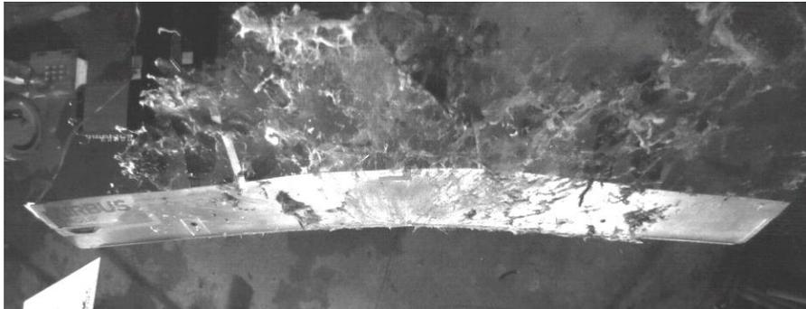
Figure 9. Maximum deflection of Krueger flap under bird impact (from high speed video).
