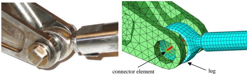
**Figure 4. Modelling of kinematic hinges.**
