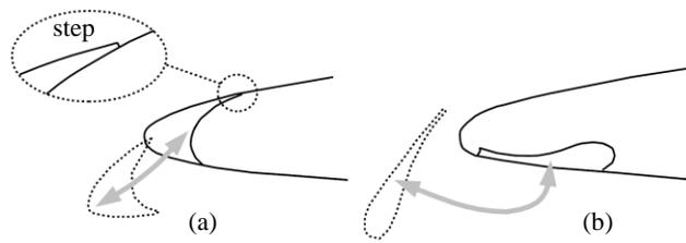
**Figure 1. Illustration of (a) conventional slat and (b) Krueger flap as wing leading edge devices.**
