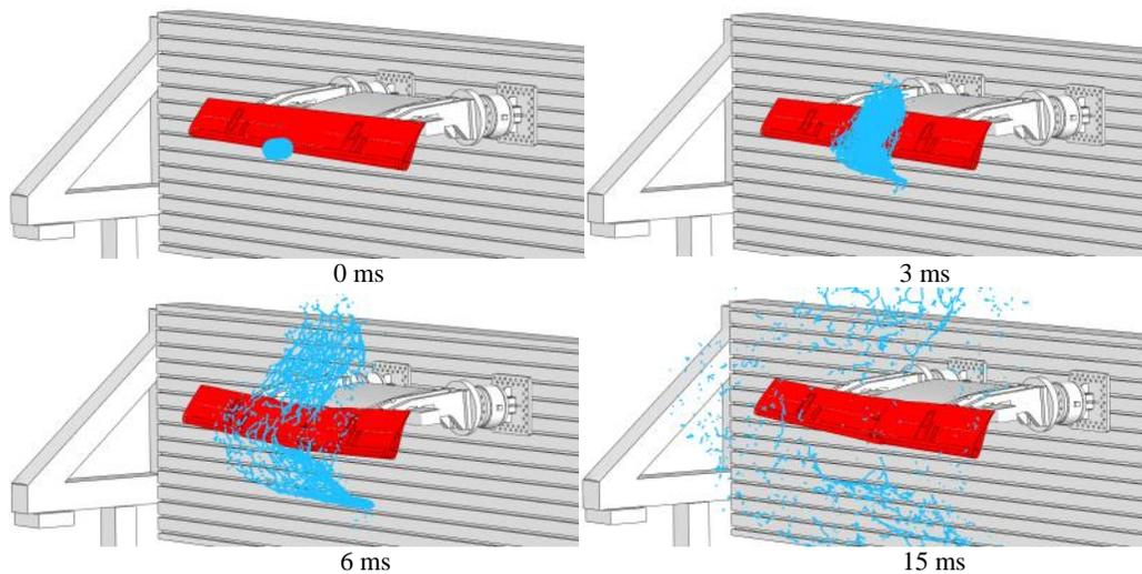
**Figure 10. Simulation of bird strike on Krueger flap including realistic test set-up.**
