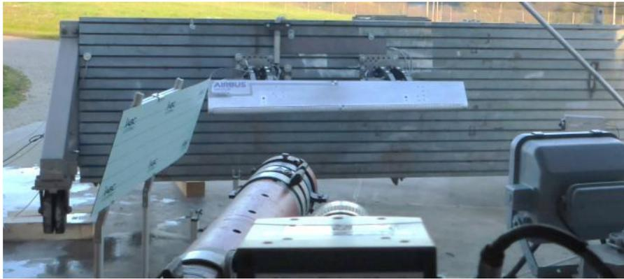
Figure 8. Full-scale bird strike test set-up with gas cannon and rigid wall.
