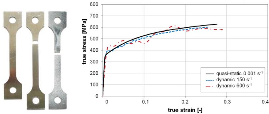
**Figure 3. Material characterization of aluminium AA 2024 for constitutive modelling.**
