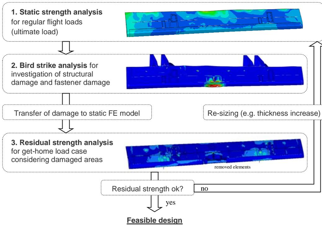
**Figure 7. Iteration loop for get-home load verification.**
